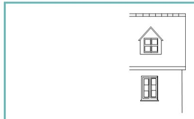
Figure 6.2: The dormer's size allows the main roof to remain the dominant feature, and the dormer window is smaller than the window on the floor below.
